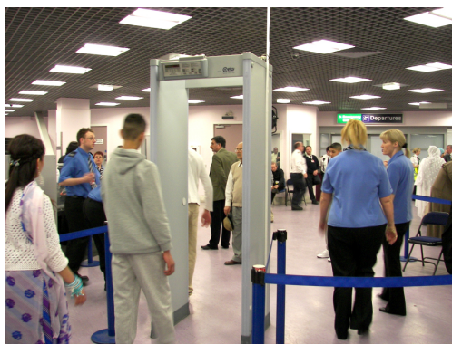
Figure 23.43 The familiar security gate at an airport can not only detect metals but also indicate their approximate height above the floor. (credit: Alexbuijds, Wikimedia Commons)
